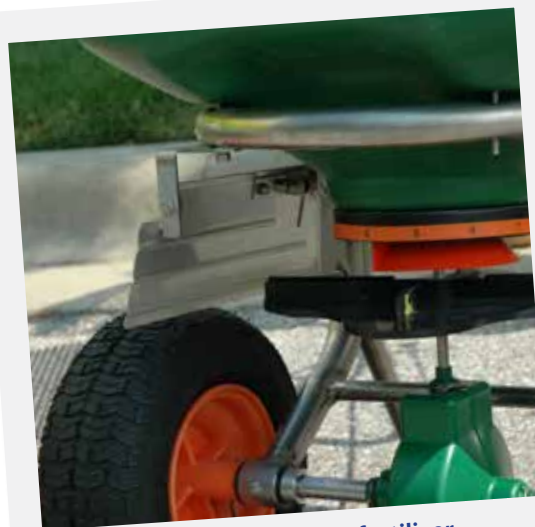
Figure 7. Broadcast fertilizer spreader with deflector attachment
