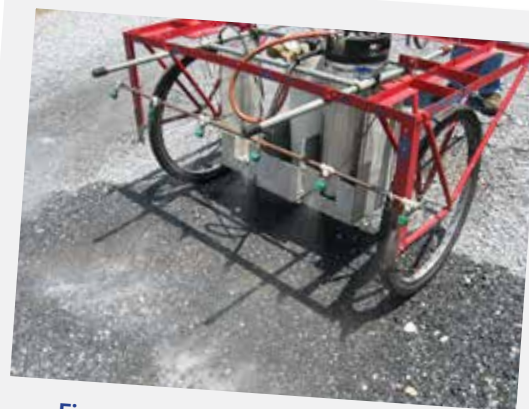
Figure 20. Evaluating nozzle and tip performance before calibration
